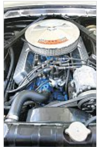
ENGINE: The much-loved 289 V8 Windsor engine.
